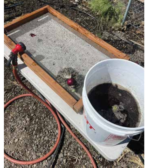
An example of our root washing station for the in-pot trial. We used a series of fine metal mesh screens to repetitively wash out the soil from the roots. This process is incredibly time consuming, but worth it for the results we found, averaging about 45 minutes per half gallon pot of soil.
